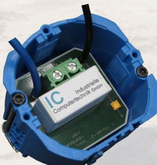
The IC power module fits even in the smallest European flush-mounted box (45 mm inside)
